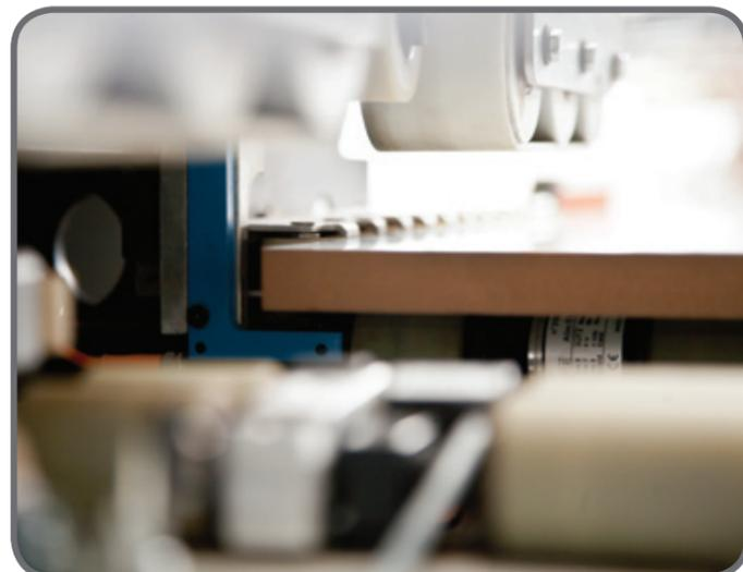
Zero setting by laser beam intervention (origin and end of the panel).
